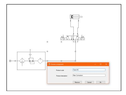
In the Properties Menu (window to the left of the drawing area), you can also assign a designation (e.g. the pipe diameter) that will be displayed near the length of the pipe involved.
